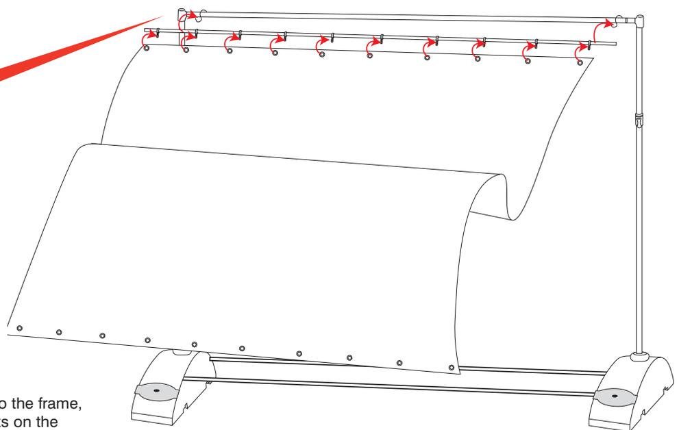
Illustration to show how graphic fits to the frame, each graphic eyelet attaches to hooks on the horizontal bungee poles.
