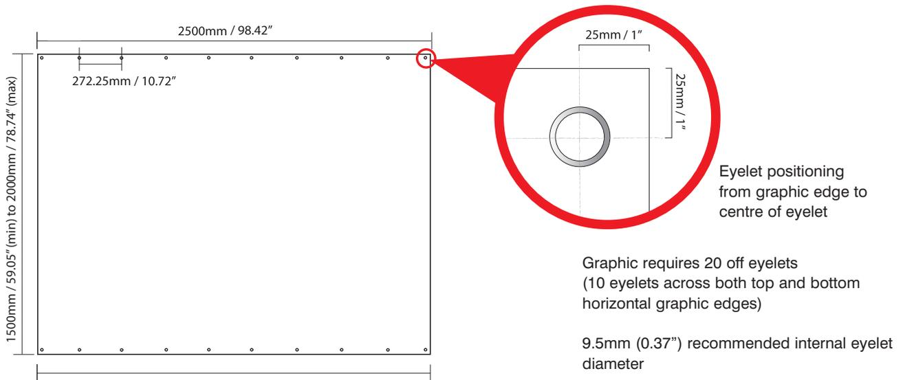
Recommended graphic dimensions and eyelet positioning
